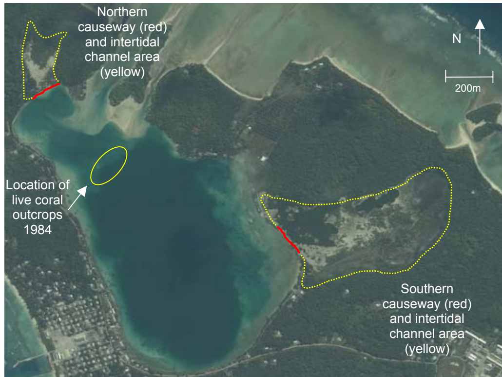
Figure 11. Water clarity in this 2004 IKONOS image of Vaitupu Lagoon is comparable to that of the 1984 airphotos and there is no indication of the lagoon becoming shallower particularly in the northern entrance area (the only significant source of transport into the lagoon). These mobile sand shoals at the entrance appear to have been surprisingly stable with few differences apparent between the 1984 and 2004 images. The absence of live coral is however evident in the northern area of the lagoon.
