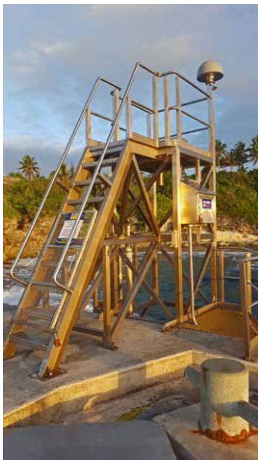
FIGURE 21. Tidal gauge located at Alofi Wharf.
